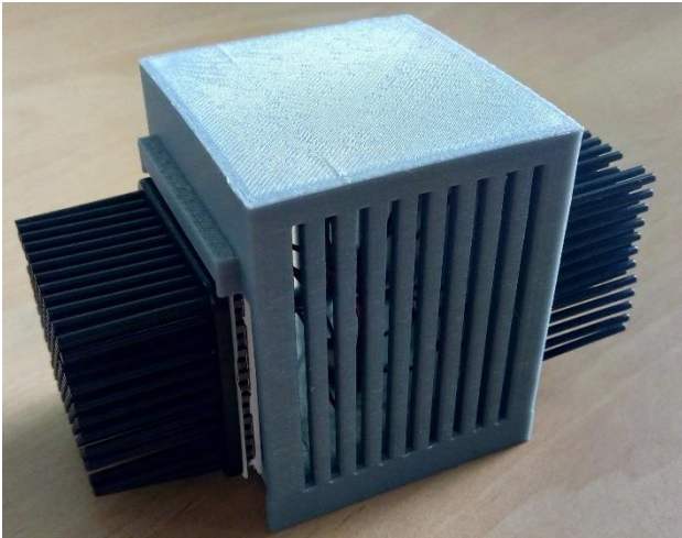
Figure 5 – Multi-sensor with U-shaped ABS plastic cover.
