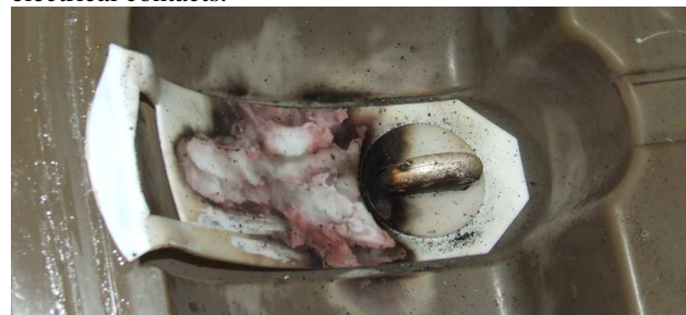
Figure 5: Pollution in the contact area with C 5 F 10 O and air gas mixture
