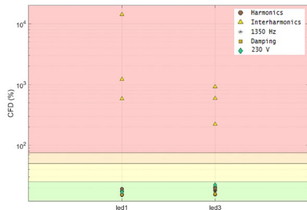
Figure 5. CFD results for LED with dimmer subjected to voltages with harmonics or interharmonics
