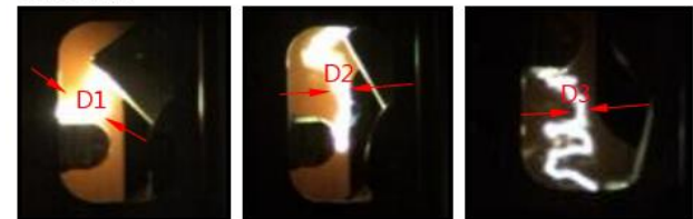
Fig. 7 The difference in the cross-sectional diameter of the arc column
