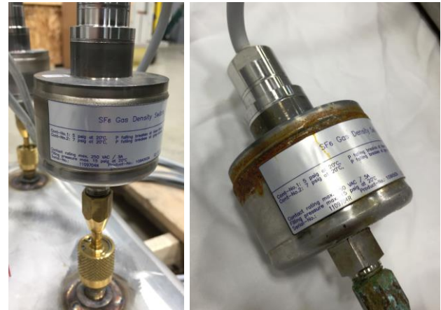
Figure 6. (Left) SF 6 Density Switch in new condition. (Right) SF 6 Density Switch with corrosion due to manufacturing processes after months of IP68 testing.
