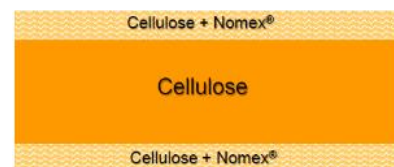
Figure 3. Schematic structure of aramid enhanced cellulose paper
