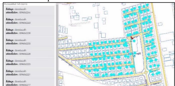
Figure 7. Tracing the location of meters linked to a transformer.
