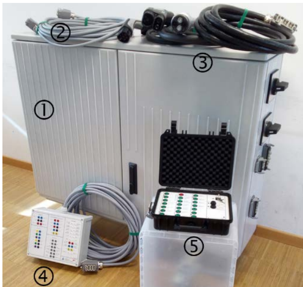
Figure 3: Measuring distribution box ① with accessories (line for remote control ②, charging power lines ③, measurement box ④, remote control ⑤)
