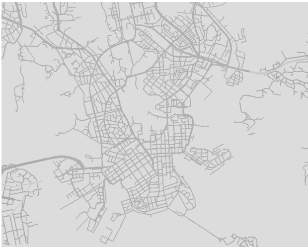
Figure 2. The relevant 10 kV area, the main peninsula of Helsinki, cropped from the original raster map. Different colors represent different unit costs and interruption related parameters. Here roads have a darker color meaning relatively lower trenching costs. All other areas are colored in lighter grey representing higher trenching costs.
