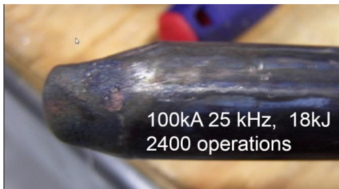
Figure 3: Modification of the arcing pin of an SF 6 interrupter due to making operations.
