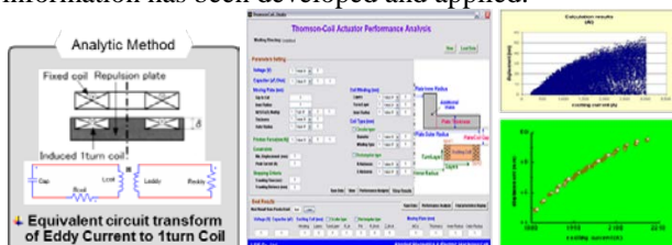
Figure 6 Equivalent Circuit Analysis S/W for Thomson Drive Mechanism (faster than FEM and similar accuracy)
