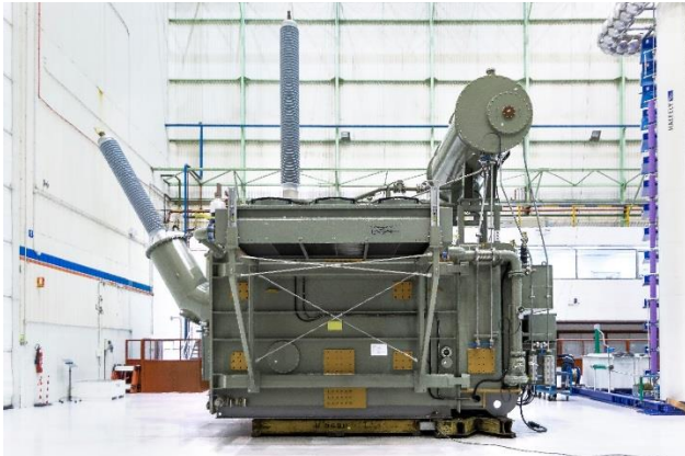
Figure 2: Transformer fully assembled during final testing
