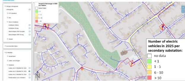
Image 5: Screenshot of Westnetz's geographic information system of Westnetz with infaded low- and medium voltage cables (basemap ©OpenStreetMap contributors)
