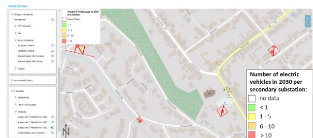
Image 4: Screenshot of Westnetz’s geographic information system with in-faded secondary substations and the predicted number of electric vehicles for each (colour); (basemap ©OpenStreetMap contributors)
