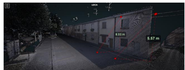
Figure 1. Example of point cloud collected through mobile mapping
