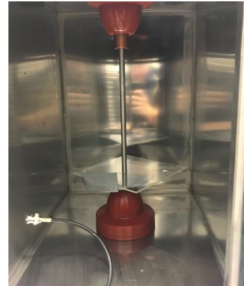
Figure 5: overview of test setup to create discharges in a demonstrational GIS (Method #2)
