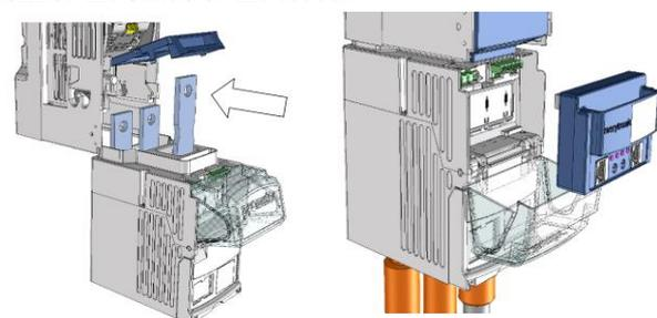
**Figure 1.** LV feeder supervisor (SAL) installation
