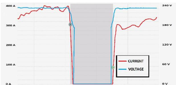
**Figure 4.** Current and voltage evolution of a blown fuse (caused by overload)
