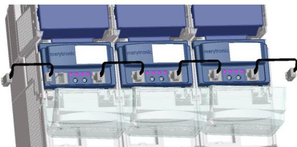
**Figure 3.** Daisy chain connection for several feeders
