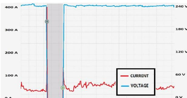
**Figure 5.** Current and voltage evolution of a blown fuse (caused by shortcircuit)
