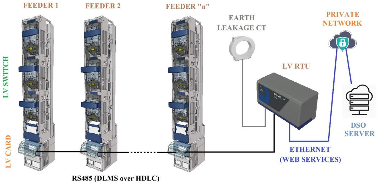
**Figure 2.** General schema for LV supervision technology
