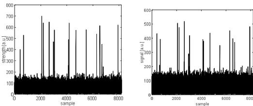
**Figure 5:** Collection of 100pC PD calibration pulses measured using two different VIS capacitive coupler.
