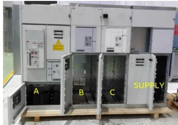
**Figure 2.** Pilot installation system showing the switchgear panels used for qualification.
