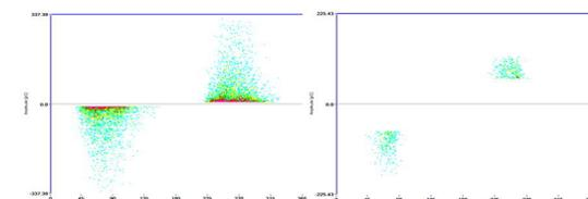
**Figure 7:** Comparison of the PD pattern without (left) and with (right) additional capacitors for the conventional PD system.
