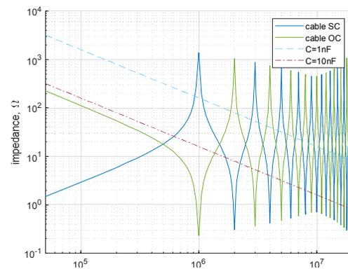
**Figure 11:** Cable impedance of a 100m long cable as a function of frequency. The results are also compared to the ones of a pure capacitor with different capacitance as used during the tests.
