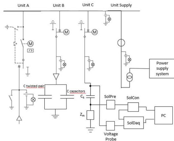
**Figure 3:** Schematic of the pilot installation including the position of the additional capacitors and the commercial PD system.
