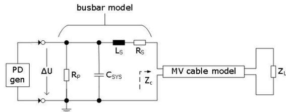
**Figure 9:** Equivalent circuit of the switchgear line-up and the attached MV cable used for the simulation.
