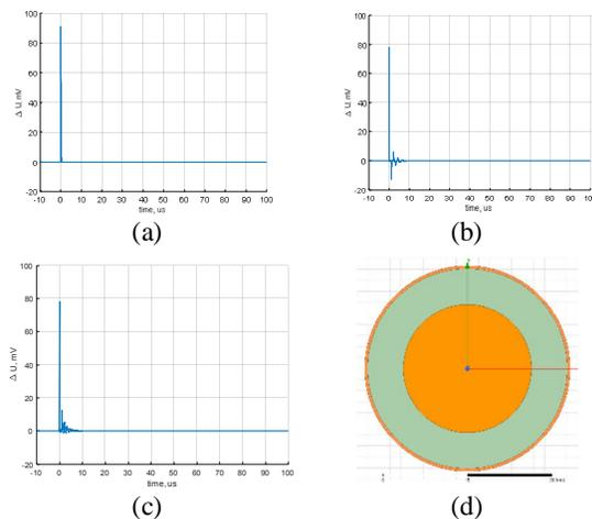
**Figure 10:** Amplitude of the pulses produced on the MV busbar corresponding to a 100pC discharge for the system presented in Figure 1 with  $C_{sys}=1$ nF. (a) no cable attached to the busbar, (b) with a 100m cable attached with a grounded end ( $Z_L = 0\Omega$ ), (c) with a 100m cable attaches with an open end ( $Z_L = \infty$ ). Subfigure (d) shows the cable geometry using for the calculation.
