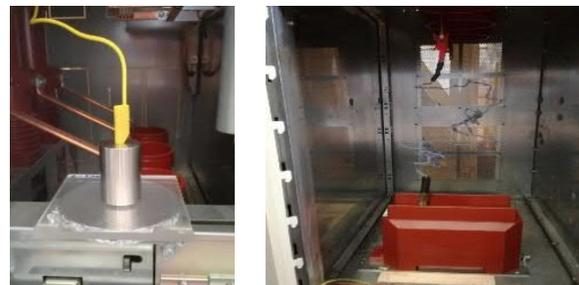
**Figure 4:** Two types of PD sources used during the qualification testing: A laboratory surface discharge producing device (left) and a current transformer rejected at acceptance test (right).
