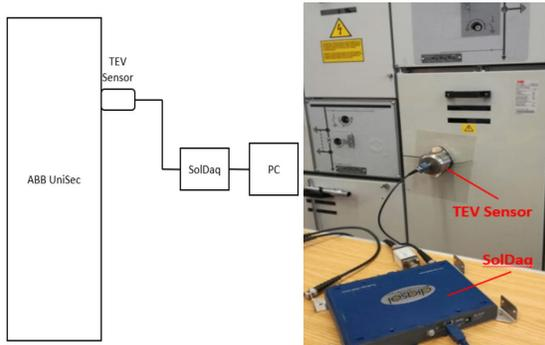
**Figure 1.** Setup of the TEV sensor, schematics (left) and photo of the real setup (right).
