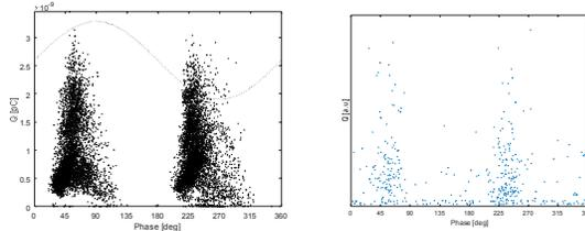
**Figure 6:** Comparison of a surface discharge pattern recorded by the commercial system (left) and with the online monitoring system (right).
