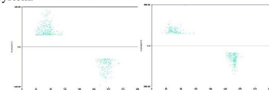
**Figure 8:** Comparison of the PD pattern without (left) and with (right) additional capacitors for the TEV sensor.
