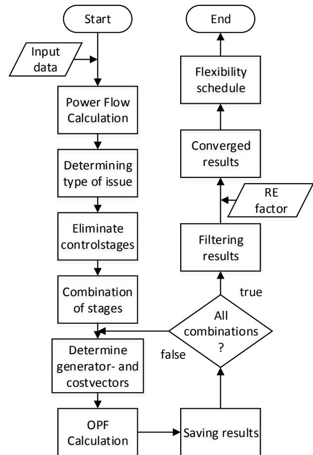
Figure 1: schematic Optimization Module process
