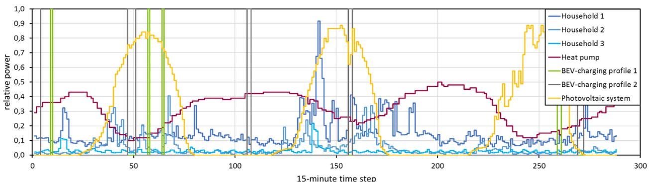
Figure 2: generic load and injection profiles of flexible systems in the urban grid
