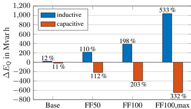
**Fig. 4:** Change in reactive energy exchange with the external grid compared to the base scenario
