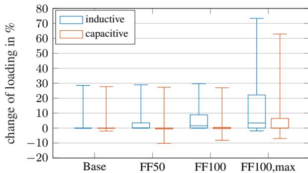
**Fig. 8:** change of equipment loading (lines and transformers) within the grid compared to base scenario
