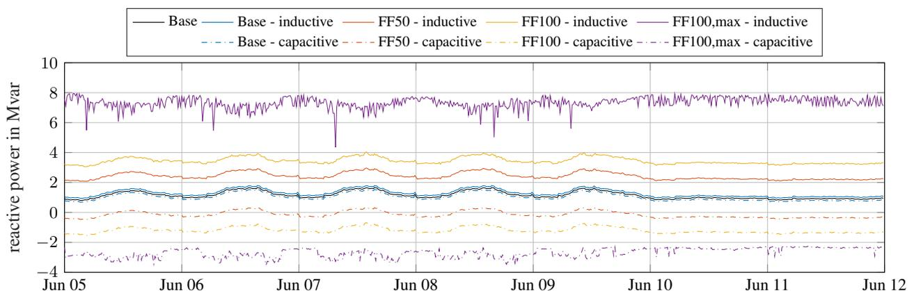
**Fig. 3:** Reactive power exchange with the external 110-kV-grid
