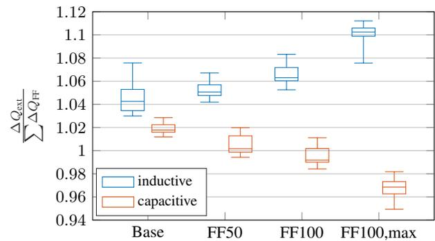
**Fig. 6:** Ratio of change of reactive power consumption of the FF-loads to the change of reactive power exchange with the external 110-kV-grid
