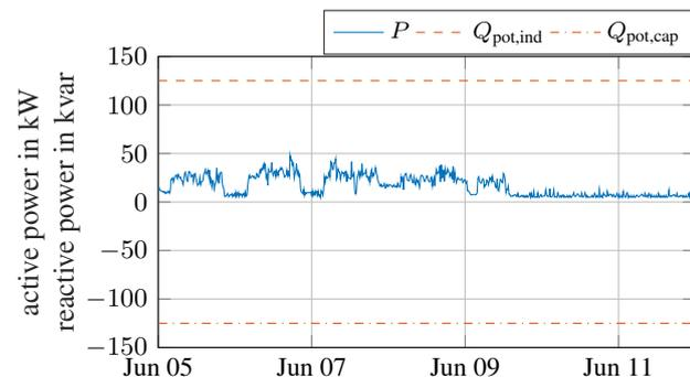
**Fig. 2:** Reactive power limits and measured active power consumption of ETA-Fabrik
