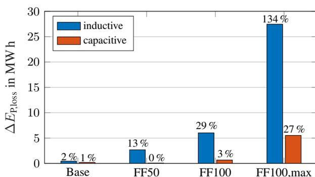
**Fig. 5:** Change in grid losses compared to base scenario
