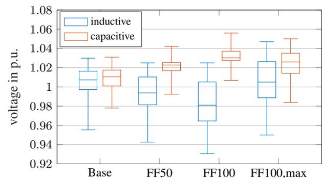
**Fig. 7:** Distribution of the voltage for all busbars within the grid
