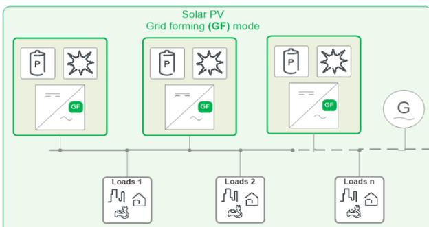
Figure 4: Grid-forming inverters with VSG technology, enabling 100% renewable penetration
