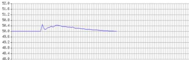
Figure 8 TUC5 - PV fluctuations on a grid formed by VSG
