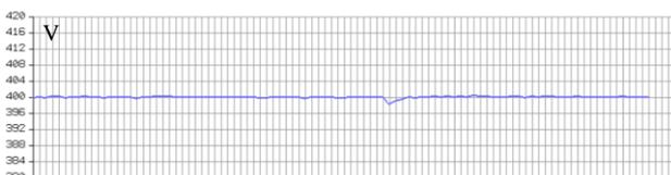
Figure 11 TUC 3 - Step load of 15 kW on grid formed by VSG
