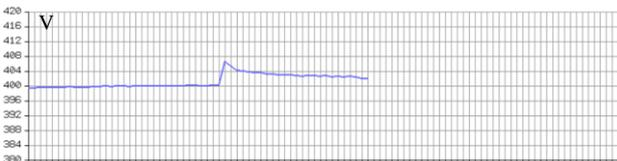
Figure 10 TUC 3 - Step load of 15 kVAR on grid formed by VSG
