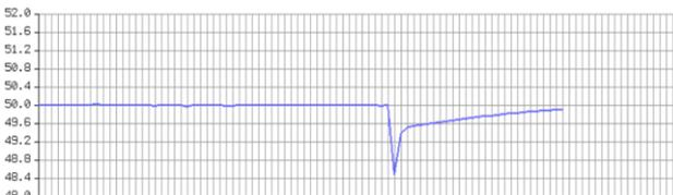
Figure 9 TUC4 - PV disconnection from a grid formed by VSG
