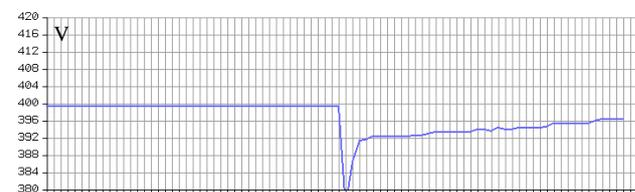
Figure 6: TUC3 - Step load of 15 kVAr (ind)
