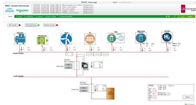
Figure 5: SPORE microgrid SCADA.
