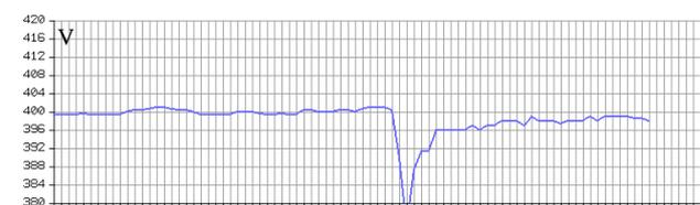
Figure 7: TUC3 - Step load of 40 kW and 30 kVAr (ind)
