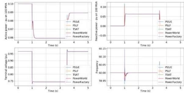
Fig. 8. Plots from Extended Voltage Sag Test
