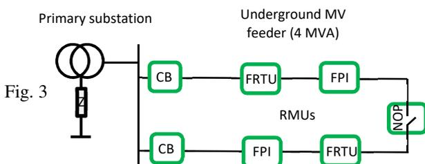
In case of a fault occurrence, the SCADA operator operates the remote controlled RMU to reconfigure the network and reduce the affected area. Then the maintenance crew dispatched on site utilizes the FPI to locate the fault:
