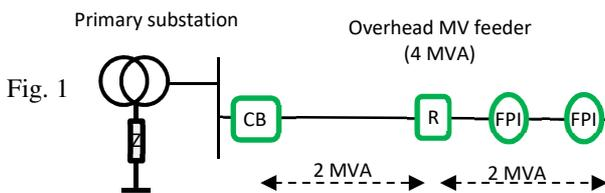
In case of fault downstream, the line recloser shall only isolate and cut power downstream. When the maintenance crew arrives on site, they will start to inspect the line from the recloser with the help of the FPI.
