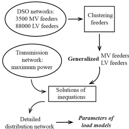
Fig. 2 Flow chart of distribution network modelling
