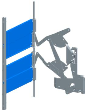
**Figure 2:** Lever system to actuate shutters
