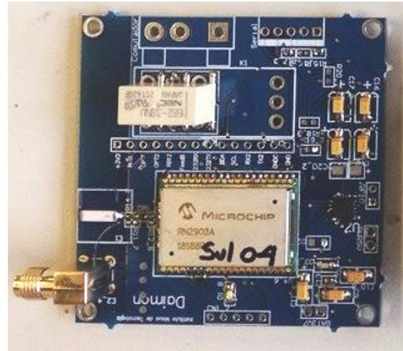
Fig. 3. Printed circuit board of communication device
