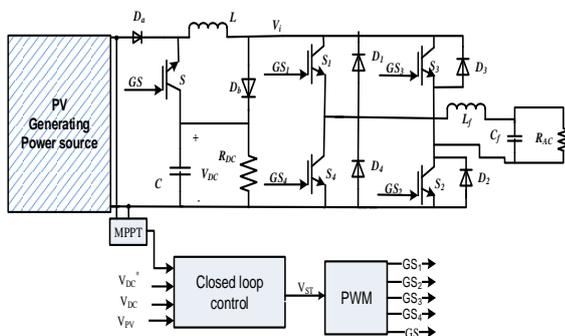
Fig.3 The circuit diagram for the SIMO-SBI
