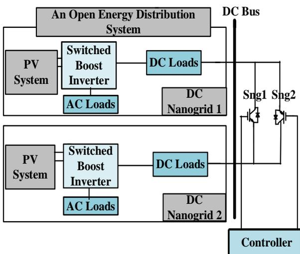
Fig.4 Two interconnected nanogrids within an OEDS
