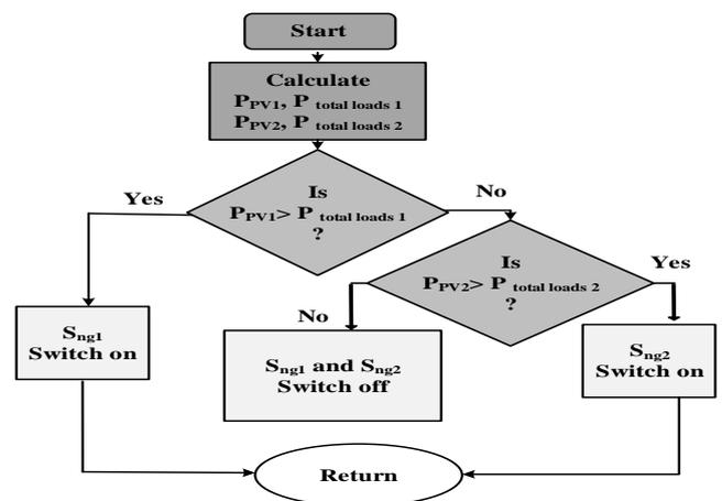
Fig.6 OEDS controller algorithm flow chart
