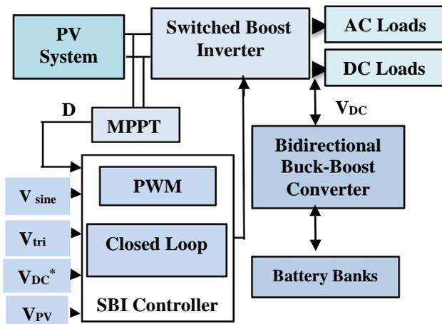
Fig.2 The DC nanogrid construction
