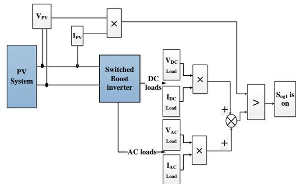
Fig.5 The controller block diagram of one DC nanogrid
