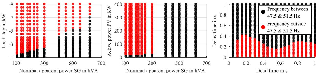
**Figure 5:** Illustration of the variation of parameters: **left)** Load Step and Nominal Apparent Power of SG, **center)** Installed Active Power PV Converters and Nominal Apparent Power of SG and **right)** Influence of Time Constants  $T_{dead}$  and  $T_{delay}$
