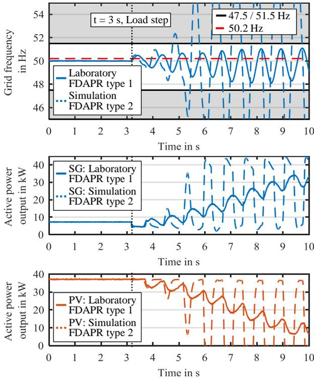
**Figure 4:** Comparison of grid frequency (top), active power output of synchronous generator (center) and PV converters (bottom) at load step of -3 kW (after 3.2 seconds) with FDAPR type 1 (laboratory) and type 2 (simulation)
