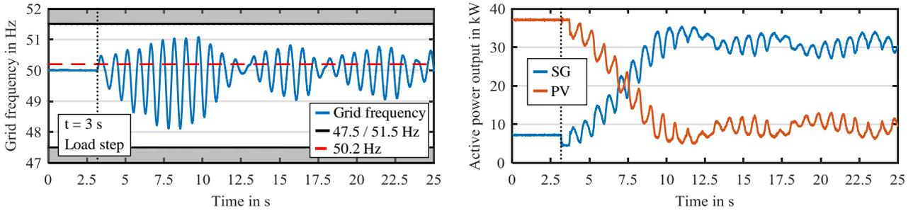
**Figure 2:** Grid frequency (left) and active power output (right) of synchronous generator and photovoltaic converters at load step of -3 kW (after 3.2 seconds) with FDAPR type 1
