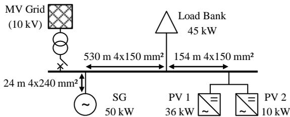
**Figure 1:** Laboratory setup for analysis of SDG characteristics
