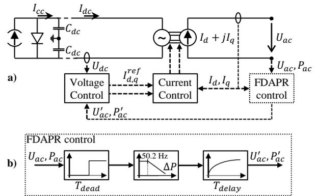
**Figure 3:** Control structure of PV converter with FDAPR
