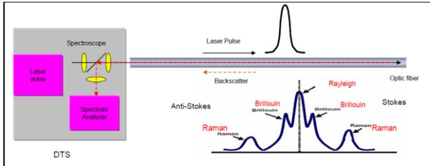
Figure 1 – DTS Utilisation of Raman Scattering
