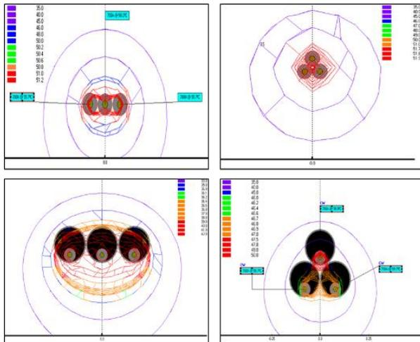
Figure 5 – CYMCAP results for heat distribution in different cable configurations
