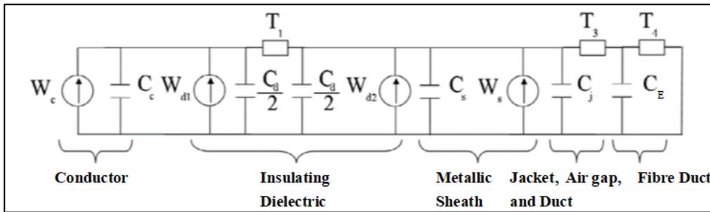
Figure 2 – Thermal Electric Analogy [7] [8]
