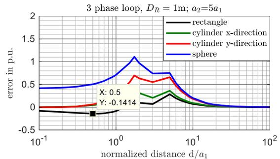
Figure 5: Error through the simplification compared to the 3D-model (negative=underestimation through simplification)
