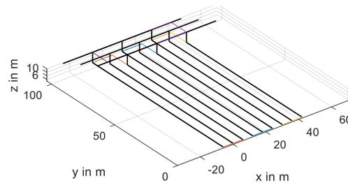
Figure 7: 3D-modell of a substation with 1 busbar and 3 branches, in color the contours of the simplified 3-loops
