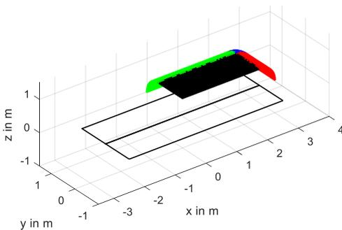
Figure 3: Part of the envelope around the loop for calculation of the maximum  $AQ$ , black: rectangle above the loop, green and red: parts of a cylinder around the outer conductor of the loop, and blue a part of the sphere, in the corner.
