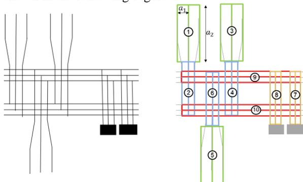
Figure 1: Plan view of a substation with 2 busbars and 5 branches, left: original plan view, right: approximation with three phase loops (1 to 10)
