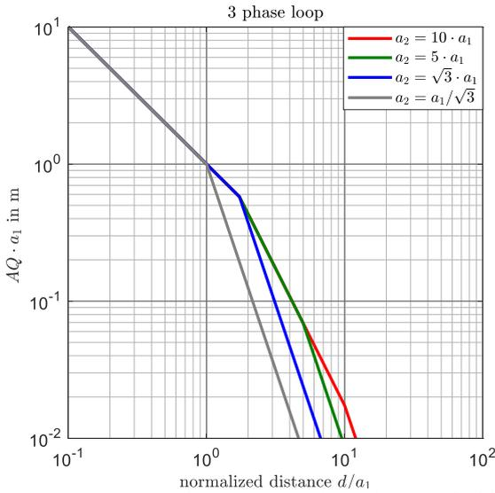
Figure 2: Action Level Quotient  $AQ$  for 3~loops with different length  $a_2$  evaluated with the simplified formulas for  $D_R=1$  m;
