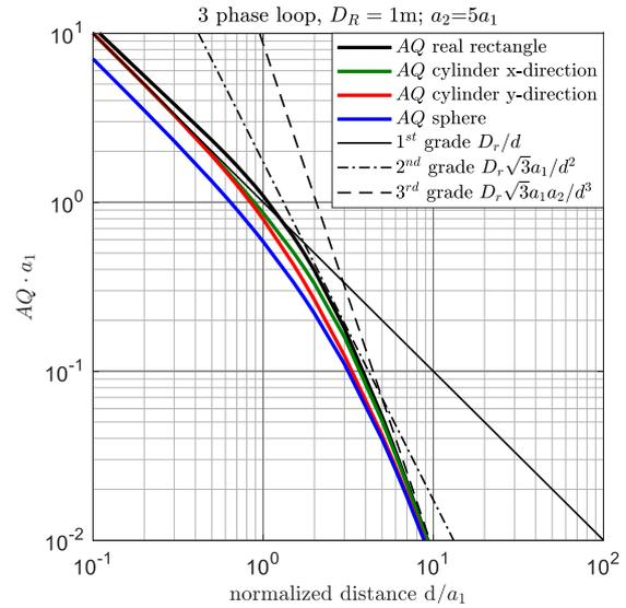
Figure 4: Maximum  $AQ$  for individual areas in a distance  $d$  for a 3~loop with  $a_2=5a_1$
