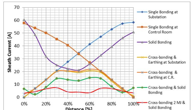
Figure 5 - Sheath current distribution for various sheath-bonding for cables of 800 mm<sup>2</sup>.
