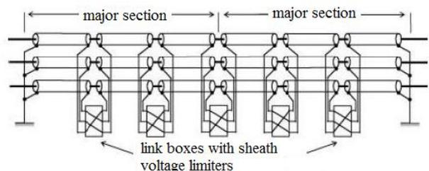
Figure 3 – Continuous cross-bonding method [4].
