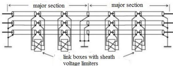
Figure 2 – Sectionalized cross-bonding method [4].
