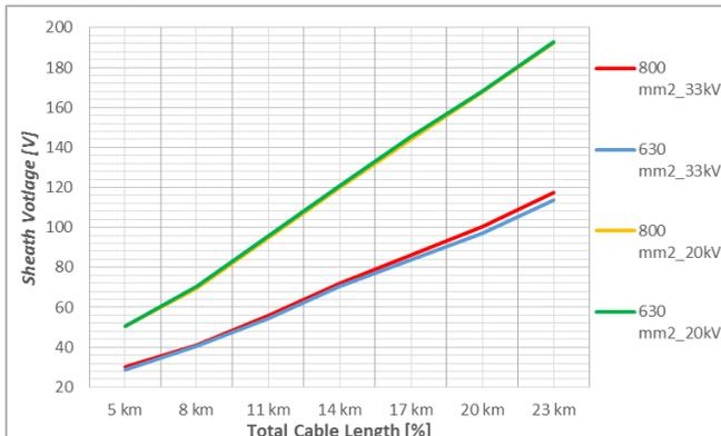
Figure 6 - Sheath voltage distribution for various cable lengths, cross-sections and voltage levels.
