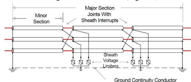
Figure 1: Implementation of cross-bonding [3].
