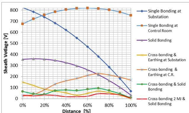
Figure 4 - Sheath voltage distribution for various sheath-bonding for cables of 800 mm<sup>2</sup>.
