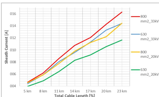
Figure 7 - Sheath current distribution for various cable lengths, cross-sections and voltage levels.
