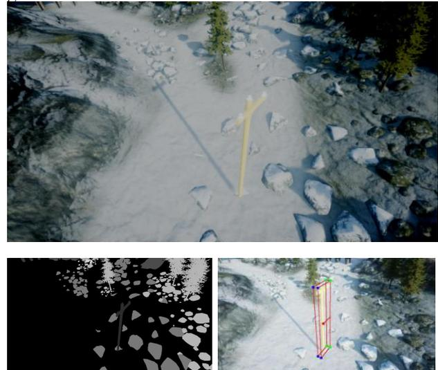
Figure 1. The Tower dataset was generated by placing 3D household object models in virtual environments. Each snapshot consists of a stereo pair of RGB images (only one of which is shown, top), pixelwise segmentation of the objects (bottom left), depth (not shown), 2D/3D bounding box coordinates (bottom right), and 3D poses of all objects (not shown).
