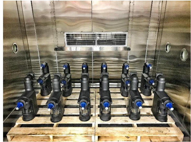
Figure 11: Modules set up in thermal chamber for extreme thermal aging (-70°C to +50°C)
