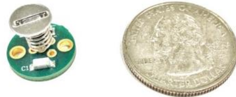
Figure 8: Miniaturized capacitive divider board to be potted into the switch module.
