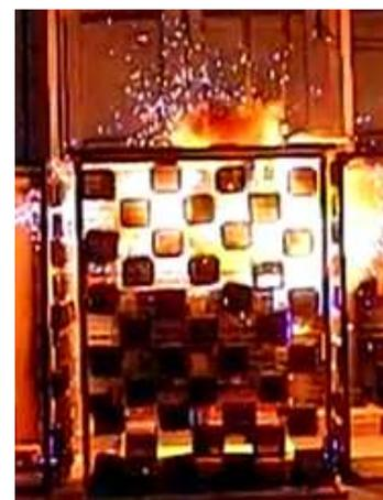
Figure 1. Internal arc test in smart LV switchgear
