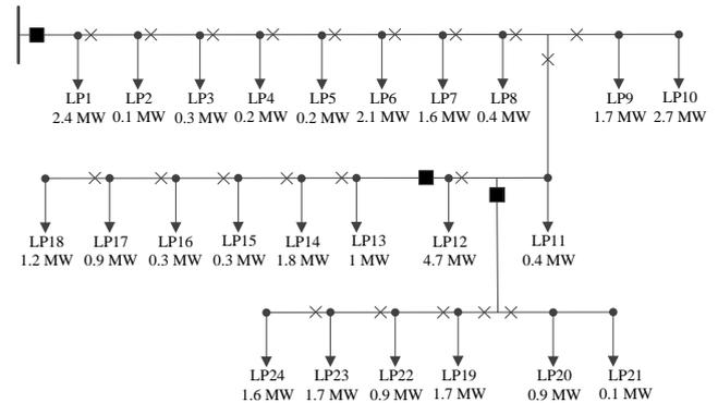
Figure 2 Single-line diagram of the test network [12]
