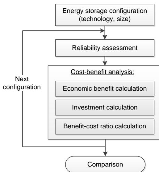
Figure 1. Flowchart of the proposed methodology for the cost-benefit analysis of energy storage in reliability studies
