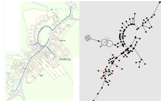
Figure 2: Example of an automated IPSA power-flow model generated from NPg's GIS database
