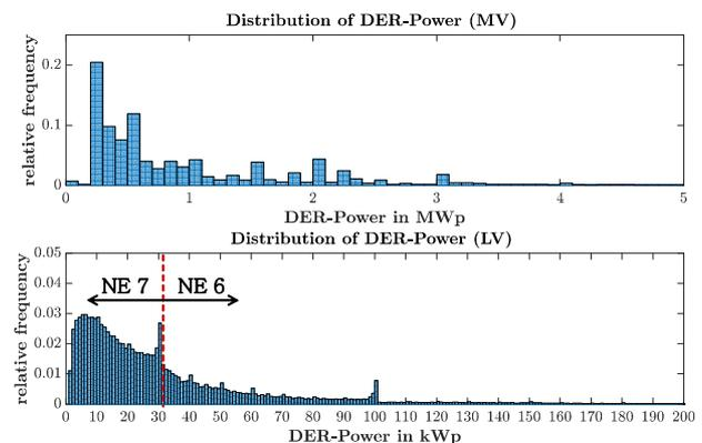
**Figure 2: Distribution function of installed DER-Power**
