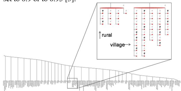
**Figure 1: Network structure of the rural grid model**
