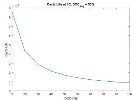
Figure 3: Cell's cycle life versus DOD
