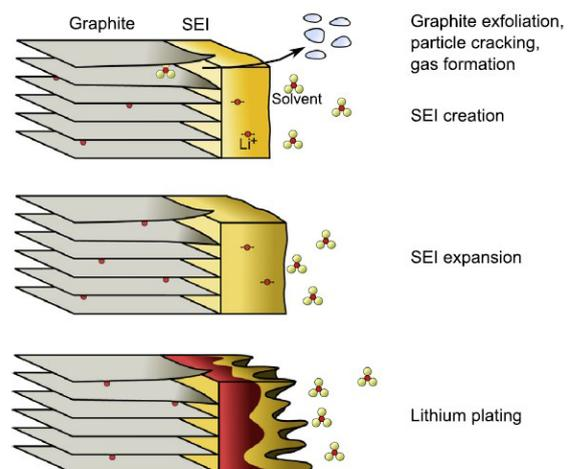
Figure 1: Ageing effects on Li-ion battery negative electrode [2]
