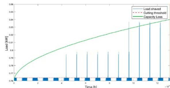
Figure 5: Example of shaving failure due to ageing
