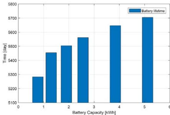
Figure 6: Lifetime of batteries versus their capacity
