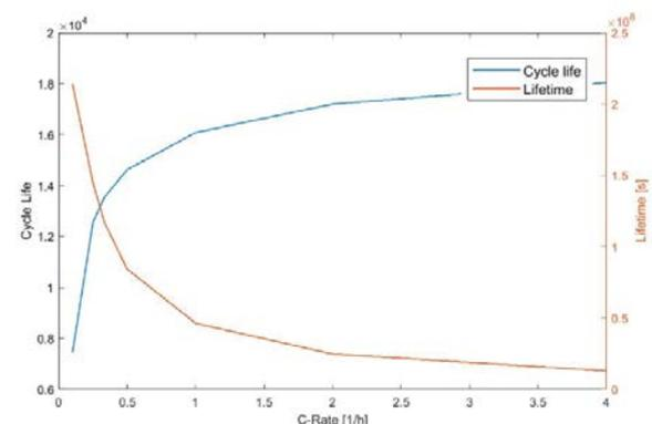
Figure 4: Cell's cycle life versus the c-rate, DOD = 40%, SOC<sub>avg</sub> = 70%
