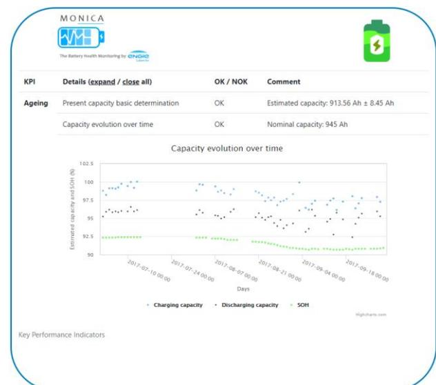
Figure 8: User interface detailed view
