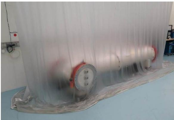
Fig. 4: Integral tightness test of a busduct in the factory.
