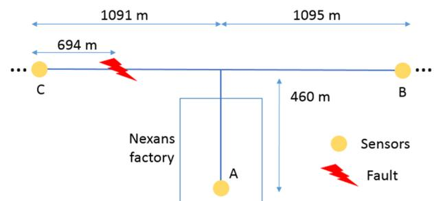
Figure 2 - NUT topology. Past Sensor B and Sensor C the network extend to other parts not covered by the system.
