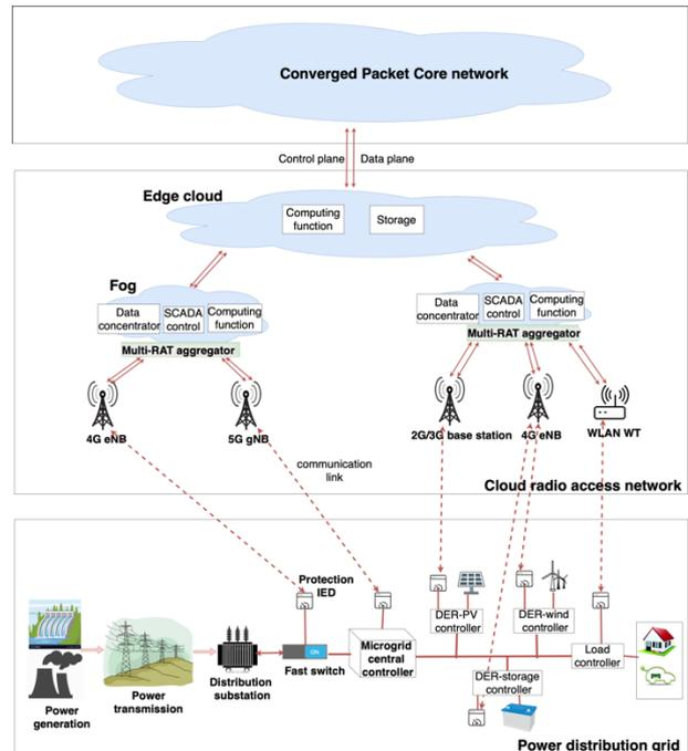
Figure 1: Proposed architecture for distribution grid operations
