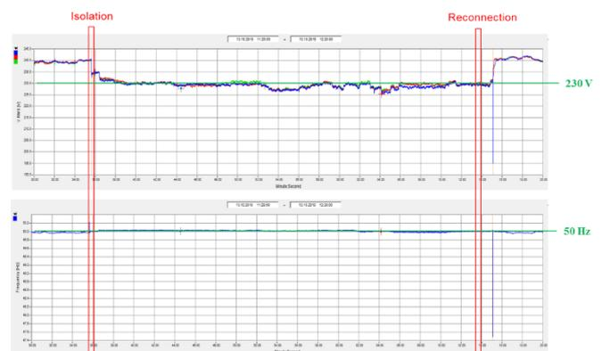
Figure 5 - Voltage (above) and frequency (bellow) measurements on LV networks during MV islanding
