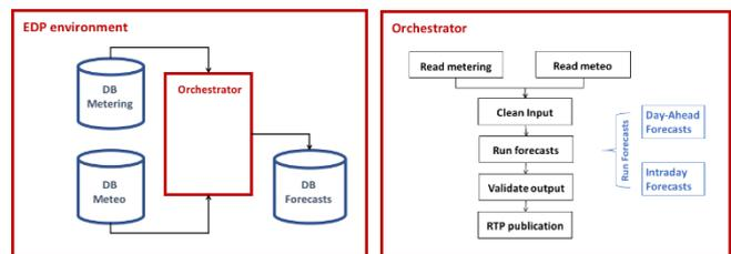
Figure 2 - Load forecasting, flow chart and modules
