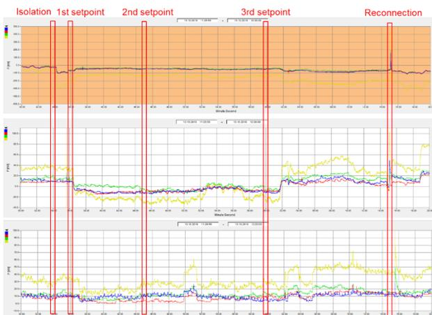
Figure 6 - Active power on ESS5 (top), LV Network 1 (middle) and LV Network 2 (bottom) during MV islanding
