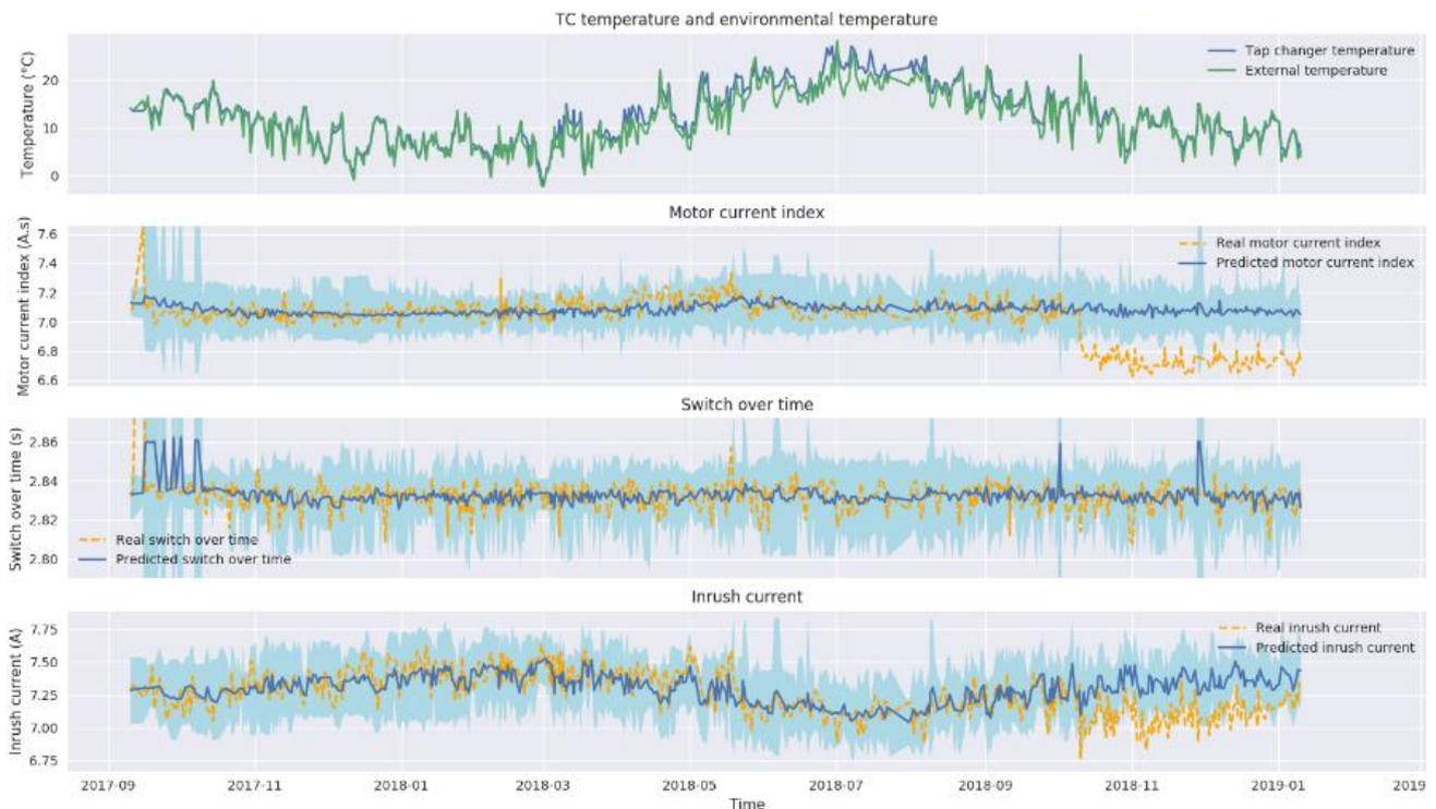
**Fig. 7** Actual data (orange line) deviates from predicted (blue line) MCI
