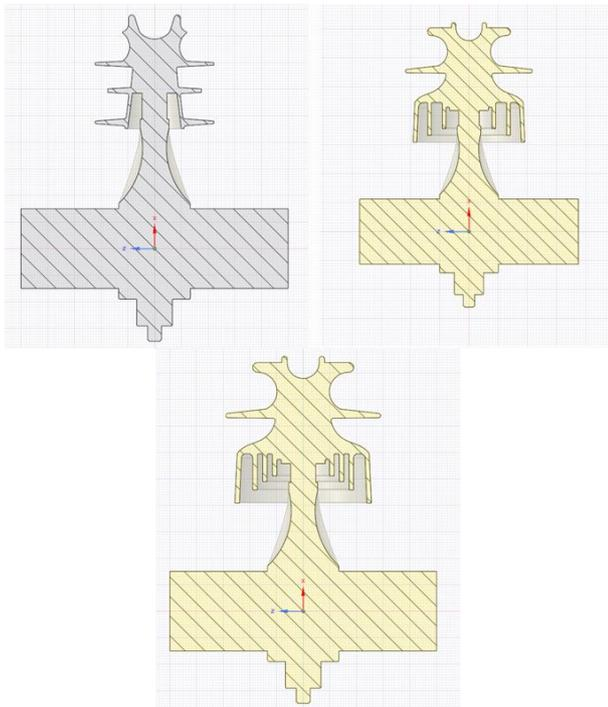
Figure 1. Pin insulator models: Conventional model (top left), 3 ribs (top right) and 4 ribs (bottom).
