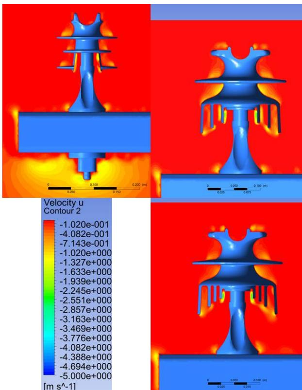
Figure 6. Velocity field over the pin insulator (negative values). Conventional model (top left), 3 ribs (top right) and 4 ribs (bottom).
