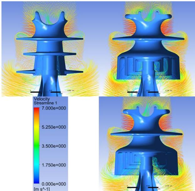
Figure 3. Streamlines over the pin insulator. Conventional model (top left), 3 ribs (top right) and 4 ribs (bottom).
