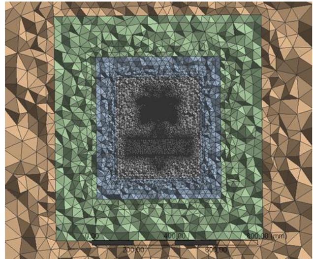
Figure 2. Variable mesh size.
