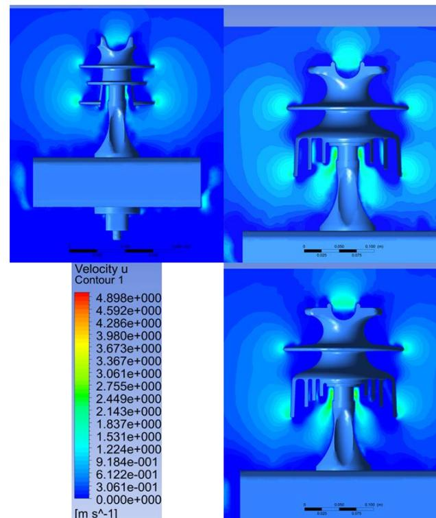
Figure 5. Velocity field over the pin insulator (positive values). Conventional model (top left), 3 ribs (top right) and 4 ribs (bottom).
