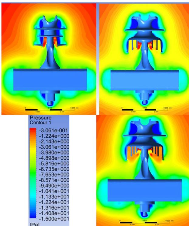
Figure 4. Pressure field over the pin insulator. Conventional model (top left), 3 ribs (top right) and 4 ribs (bottom).
