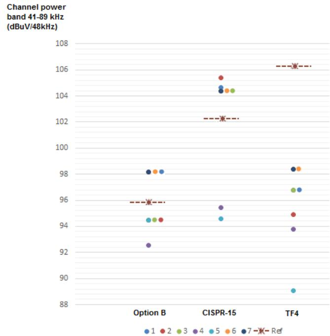
Figure 6. Minimum channel power of noise in band 41-89 kHz required to fail the communications for each of the considered meters (1-7). The channel power value of the noises adjusted to the curves (Option B, CISPR-15 and TF4) is defined as “Ref”.
