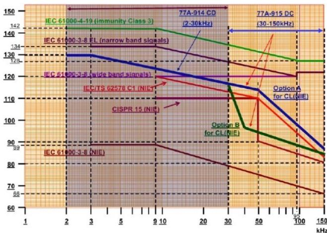
Figure 1. Different EMC standards and limits for emissions from electronic equipment [7].
