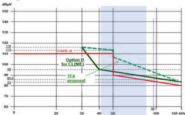
Figure 4. Considered emissions for the tests. The blue zone corresponds to the frequency band of interest (41-89 kHz).
