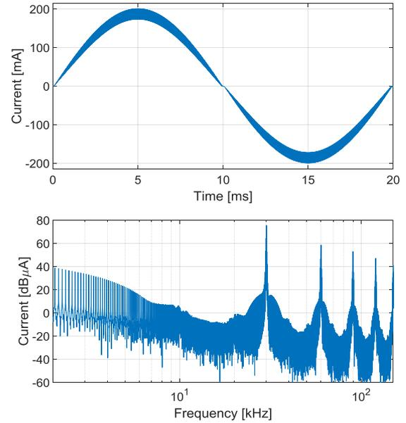
Figure 5 Grid current obtained with the complete model without taking into account the EMI filter. Time domain over 1 period (above) and frequency domain computed over 10 periods (below).
