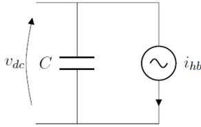
Figure 4 Half-bridge simplification
