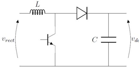
Figure 3 Active Power Factor Correction
