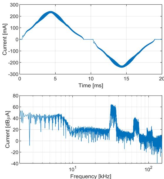
Figure 7 Measurements results of the current taken by the CDE-053 fed by a programmable voltage source. Time domain over one period (above) and frequency domain computed over 2 periods (below)
