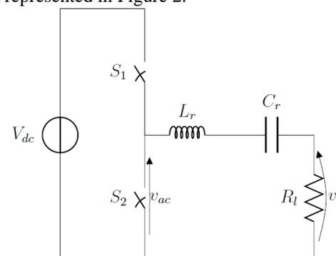
Figure 2 DC-AC converter and lamp
