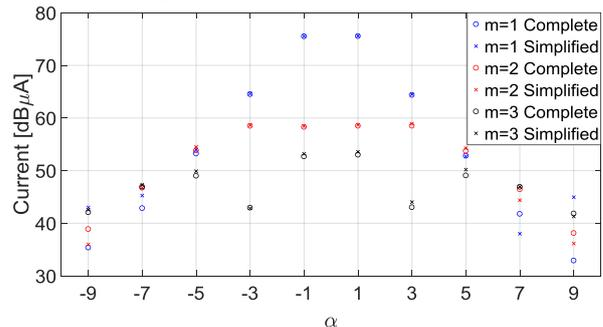
Figure 6 Comparison of the grid current harmonics magnitude obtained with the complete model and the simplified model
