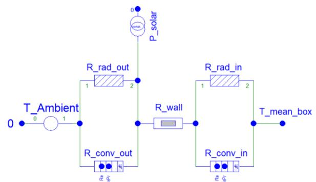
**Figure 2.** Thermal network model.
