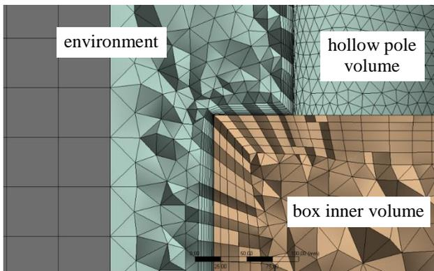
**Figure 4.** Detailed view on meshing.
