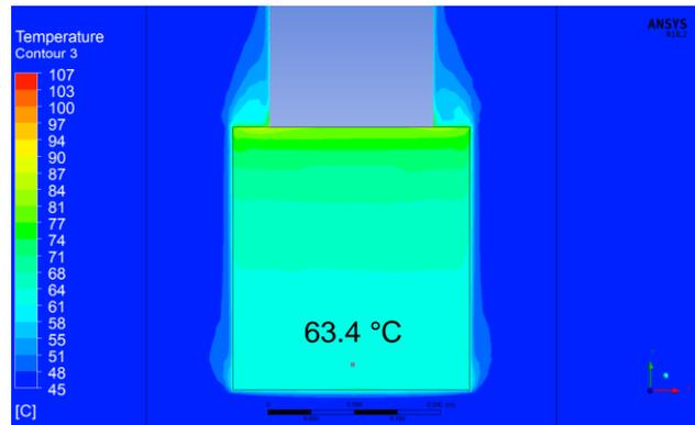
**Figure 5.** Contours of temperature field – Dubai.
