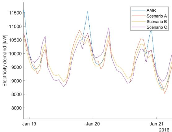
Figure 4. Case area load curve during wintertime peak load with different load control scenarios.
