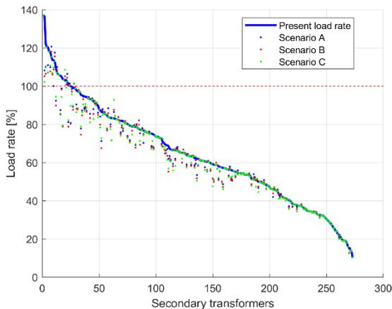
Figure 12. Secondary transformers' load rate with different load control scenarios and PBT.
