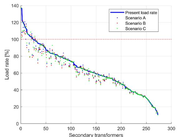
Figure 7. Secondary transformers' load rate change with different load control scenarios.
