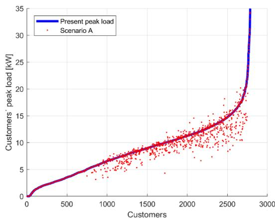
Figure 5. Customers' original peak load and peak load with load control scenario A.
