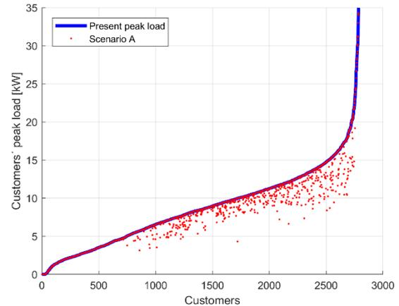
Figure 9. Customers' peak load before and after load control scenario A in case of PBT.
