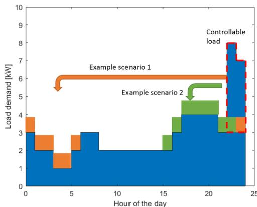
Figure 1. Basic example of controllable nighttime load and load control. Example scenario 1 means that evening controlled load is distributed to that night more evenly, not to previous morning.
