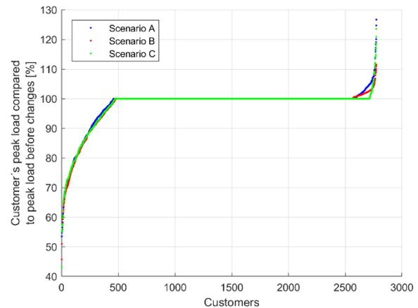
Figure 6. Relative change in customers' peak load with different load control scenarios.
