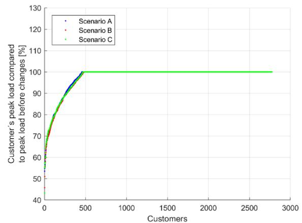
Figure 10. Relative change in customers' peak load with different load control scenarios in case of PBT.
