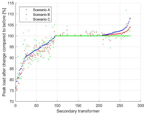
Figure 8. Change in secondary transformers' peak load without customer side peak load limitation
