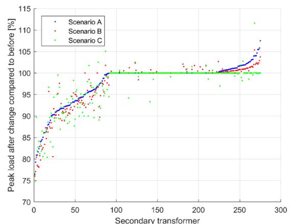
Figure 11. Relative change in secondary transformers' peak load with different load control scenarios and PBT.
