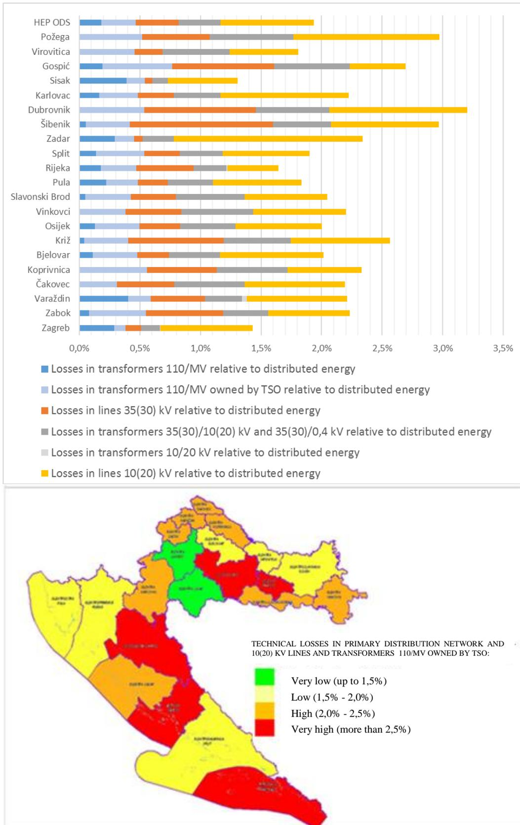
**Figure 3.** Technical losses in the primary distribution network and 110/MV transformation owned by transmission system operator and 10(20) kV network relative to distributed energy
