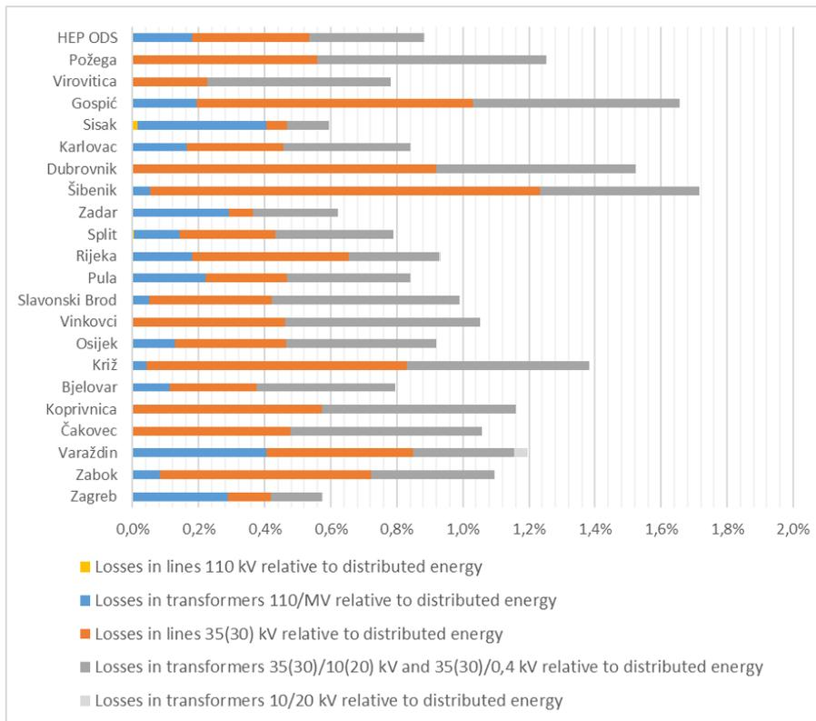
**Figure 1.** Technical losses in primary distribution network relative to distributed energy
