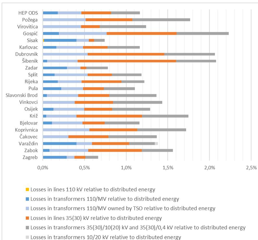
**Figure 2.** Technical losses in primary distribution network and transformation of 110/MV owned by transmission system operator relative to distributed energy
