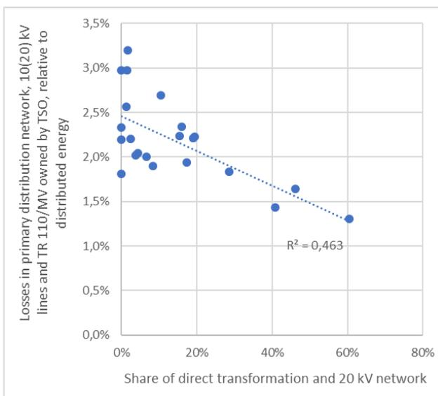
**Figure 4.** Technical losses in primary distribution network and transformation of 110/MV owned by transmission system operator relative to distributed energy
