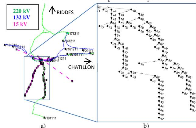
Figure 2: The integrated MV/HV/EHV grid: (a) map of the MV feeders and of surrounding HV grid, (b) the one-line diagram of the two feeders
