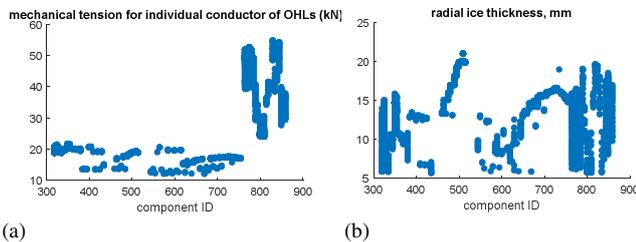
Figure 3: Mechanical tension (a) in kN, and wet snow sleeve thickness (b) for MV and HV lines, scenario S1 moderate wet snow
