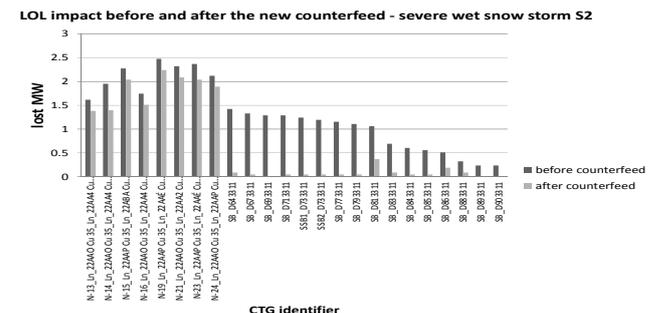
Figure 6: Bar diagram of the LOL impact of the contingencies before and after the new counterfeed, severe wet snow event S2
